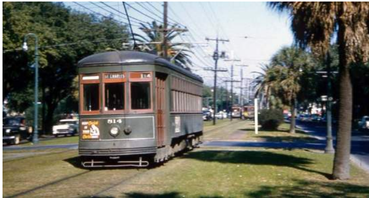
Grass Trackbed in New Orleans
