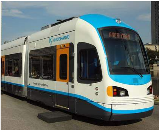
Battery/Ground Level Power Supply Modern Streetcar
