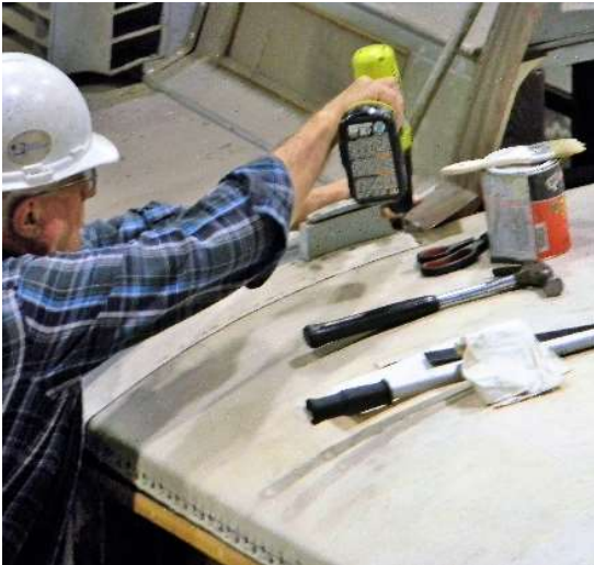
NOT SO FAST! On this job, there are ALWAYS one or two more tasks that need to be done. Here, Jim pre-drills for the necessary canvas strips which will cover the gaps between the bonnet roof and the main car body.
