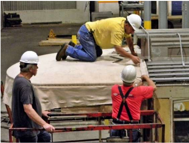
The inboard transverse edge of the canvas is fitted and secured.
