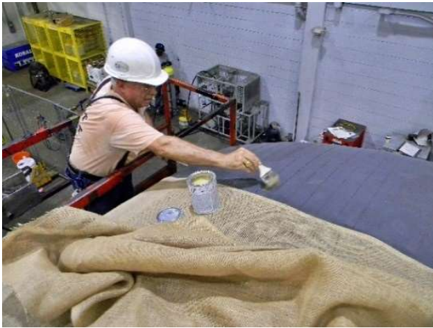
Similarly, back at the "B" end, Jim lays down a strip of cement to secure the burlap in place during the overlaying of the canvas to come. Thus, will a wrinkle-free outcome be assured.
