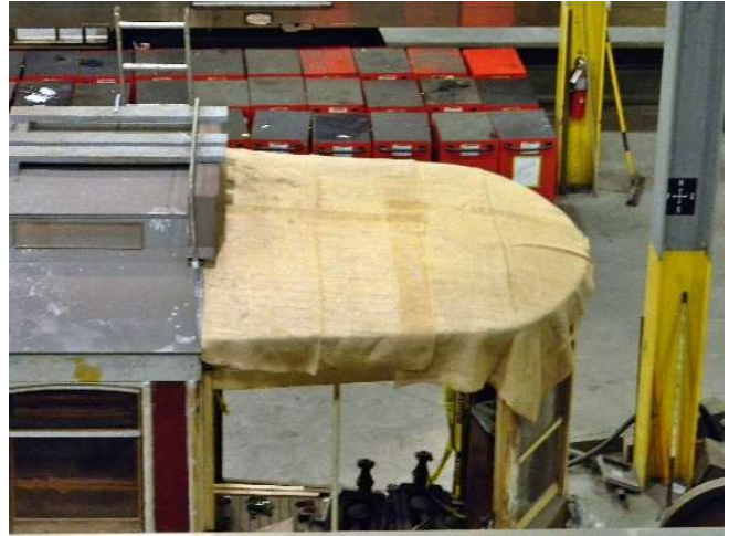
Underlayment is in place.
