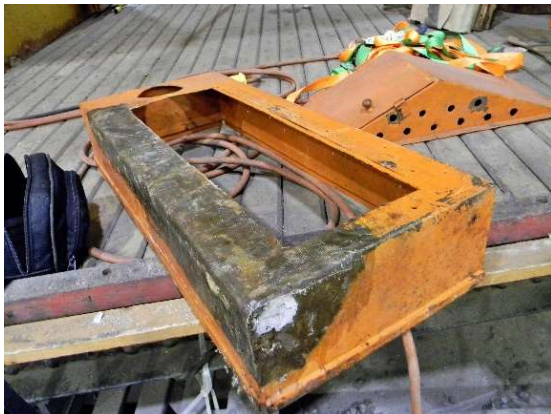
The destination sign box from the "B" end had suffered what many diagnosed as terminal rust-away. But, Doctor Bob Hooper to the rescue! Bob removed the dead "tissue" and skillfully regenerated new "flesh" using fiberglass and epoxy resin. Where do we find such people? We could use a few more, if you're out there!
