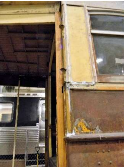
Teamwork gets 'er done! NOTE: The only place on the car where sheet metal sheathing rust out was repaired with a fiberglass / epoxy patch. (Circa 1976 at Ringoes).
