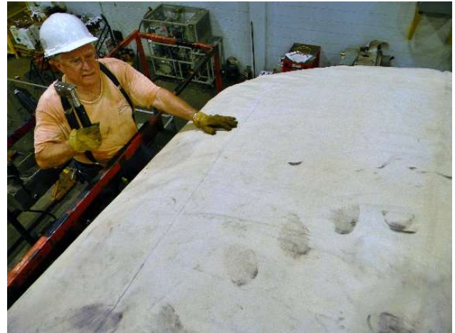
Canvas is laid on the "B" end, and neatly done! Except for Quasimodo's dirty footprints
